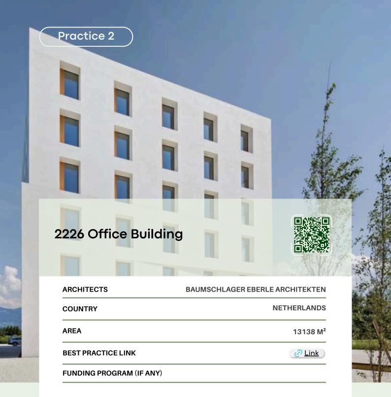
The '2226' office building maintains a year-round indoor temperature of 22–26°C without traditional HVAC systems. Its thick insulated brick walls, high ceilings, and automated windows allow occupant and equipment heat to suffice. This passive design cuts heating energy use by about 80% compared to similar offices.
